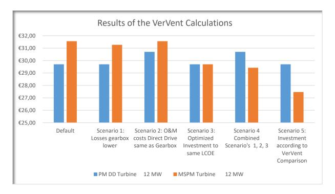
An increase in the O&M costs of the direct drive turbine, due to a larger ring generator and heavy load on the MBU) certainly increases the LCOE of this turbine. The increase used in the analysis is not yet sufficient for an LCOE comparable to that of the gearbox turbine; the latter continues to hold a higher LCOE.
