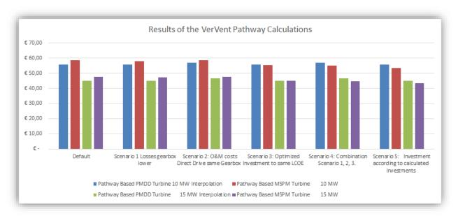
In scenarios 4 and 5 of the Pathway Calculations the LCOEs of the gearbox turbine are lower than those of direct drive. But that does not necessarily mean that the gearbox turbines makes more profit. Because the system losses of the direct drive turbine are lower than those of the gearbox turbine, the efficiency is higher and thus the turnover.
